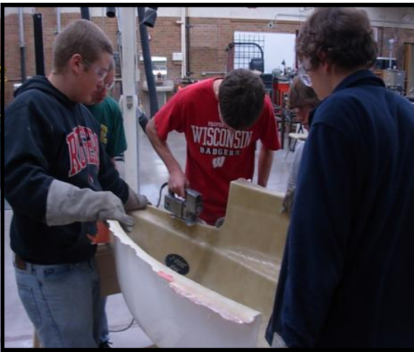
George, Zach, Kieran, and Branden work on preparing the body for painting.
