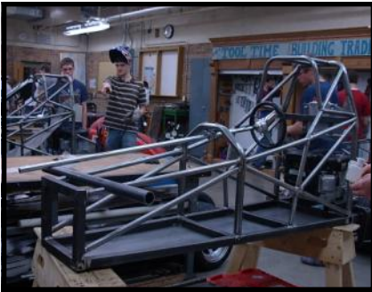
Our chassis completely welded along with back end attached.
